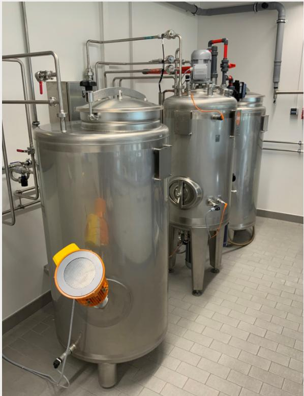
200-L ACETATOR pilot plant according to industrial standards
