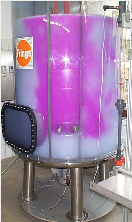
Test tank for pilot scale mixing tests
