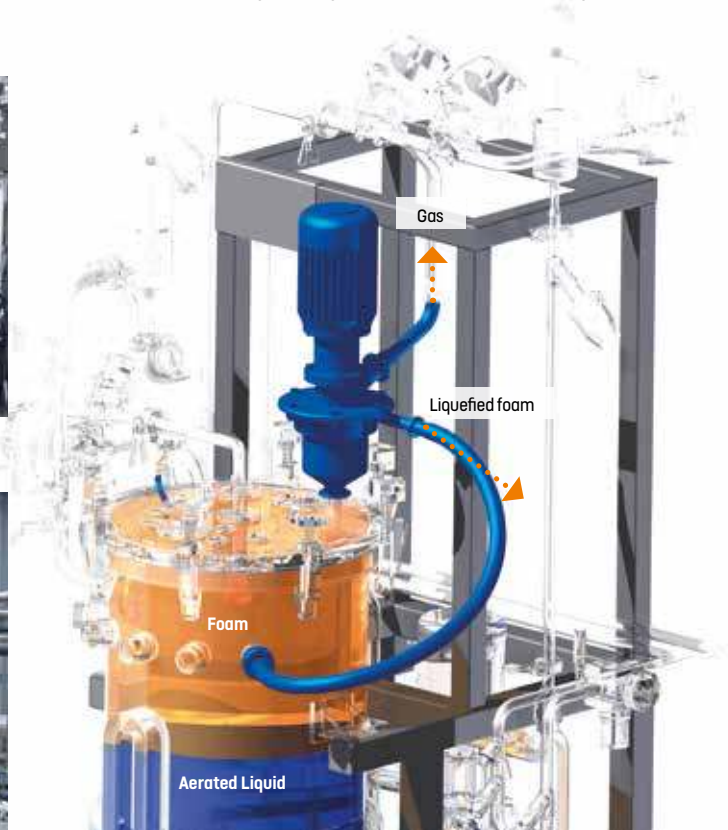
Functional Sketch of a FOAMEX on the Head of a Pilot Scale Bioreactor
